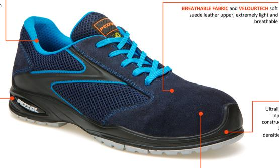
Ultralight and flexible TYRE PU/PU sole thanks to Smart Injection: this special technology combines the mold construction with the injection process of the PU Esolight 2.0 compound and allows to achieve different PU-densities guaranteeing lightness, flexibility and durability
